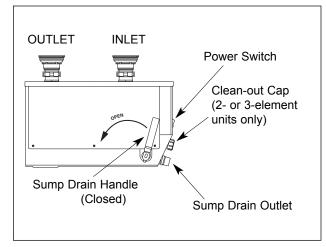
Figure 10. Hydro-Heater Side View
